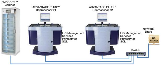
In this configuration, the Medivators devices are incorporated into the facility network, primarily to back up the databases to a network share.
