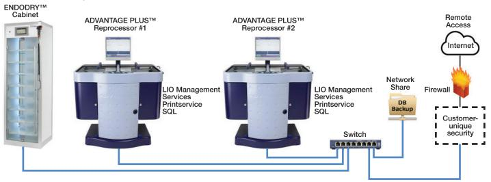
This configuration adds one item to the Option 3 configuration: Internet connection for BeyondTrust remote access. Remote access allows a Medivators Technical Support Representative to connect to the PC to assist the operator with LIO-related questions, to troubleshoot problems, or to install Medivators software updates. An Internet connection for remote access requires that the facility IT department implement security as they see fit. See *Additional Information* section for more information.
