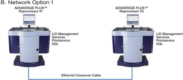
Connecting an Ethernet crossover cable between two ADVANTAGE PLUS™ Reprocessor PC's is the most basic form of network.
